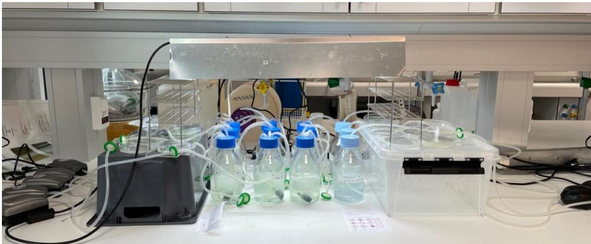
Figure 22 - Picture of the overall setup. The flasks were maintained under constant light and air supply, allowing for the growth of microalgae cultures.
