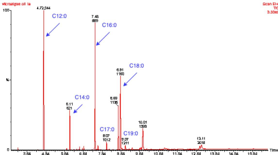
Figure 37- Chromatogram revealing the FAME composition of microalgae oil extracted from PBR1.
