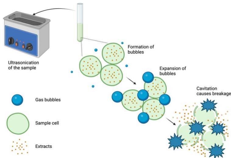
Figure 12 - Visual representation of the process of ultrasound-assisted extraction created with Created with BioRender.com and inspired from [129].
