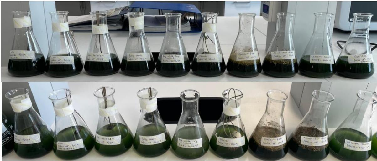
Figure 50 - Sedimentation, flocculation tests. Upper picture taken the day of inoculation; lower picture taken 3 days later.
