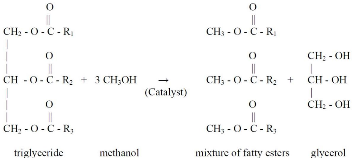
Figure 6 - Transesterification process to biodiesel from [53].
