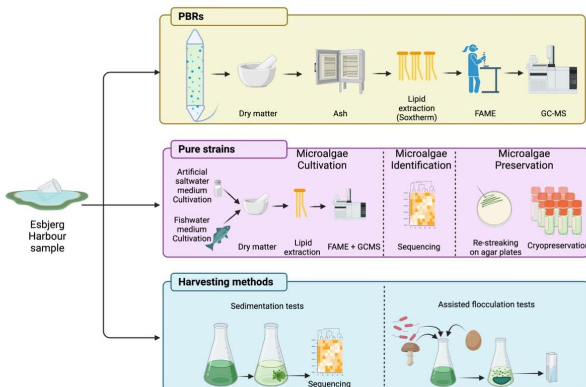
The first phase of the laboratory work in this master thesis involved cultivating a large amount of biomass inside 2L photobioreactors. Gravimetric methods, Fatty Acid Methyl Ester (FAME) analysis, and Gas Chromatography-Mass Spectrometry (GC-MS) were used to characterize parameters such as dry matter, ash content, and lipid content.
