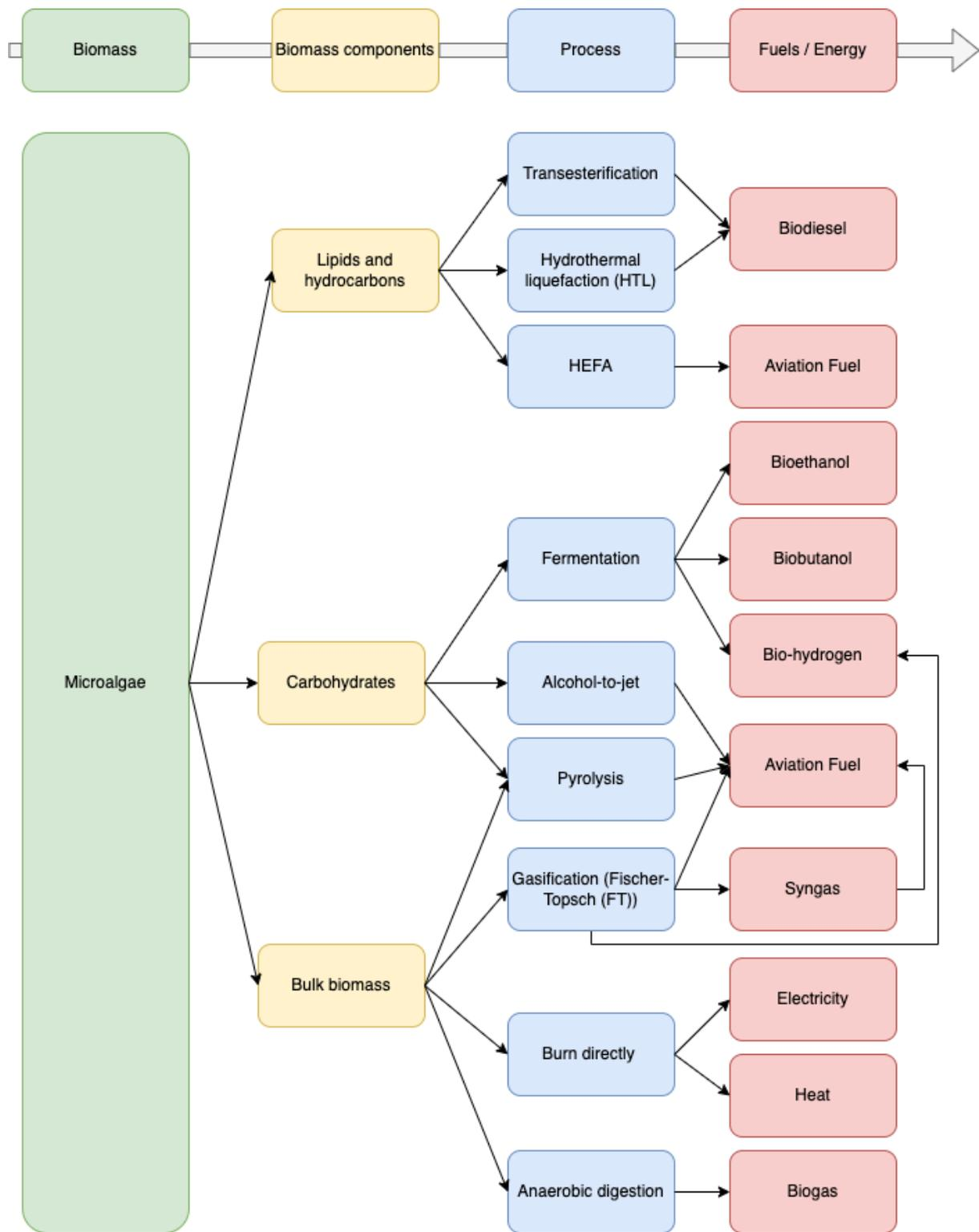
Figure 7 - Routes for microalgae production figure adapted from Hoang et al. 2022 [17], [54], [55].
