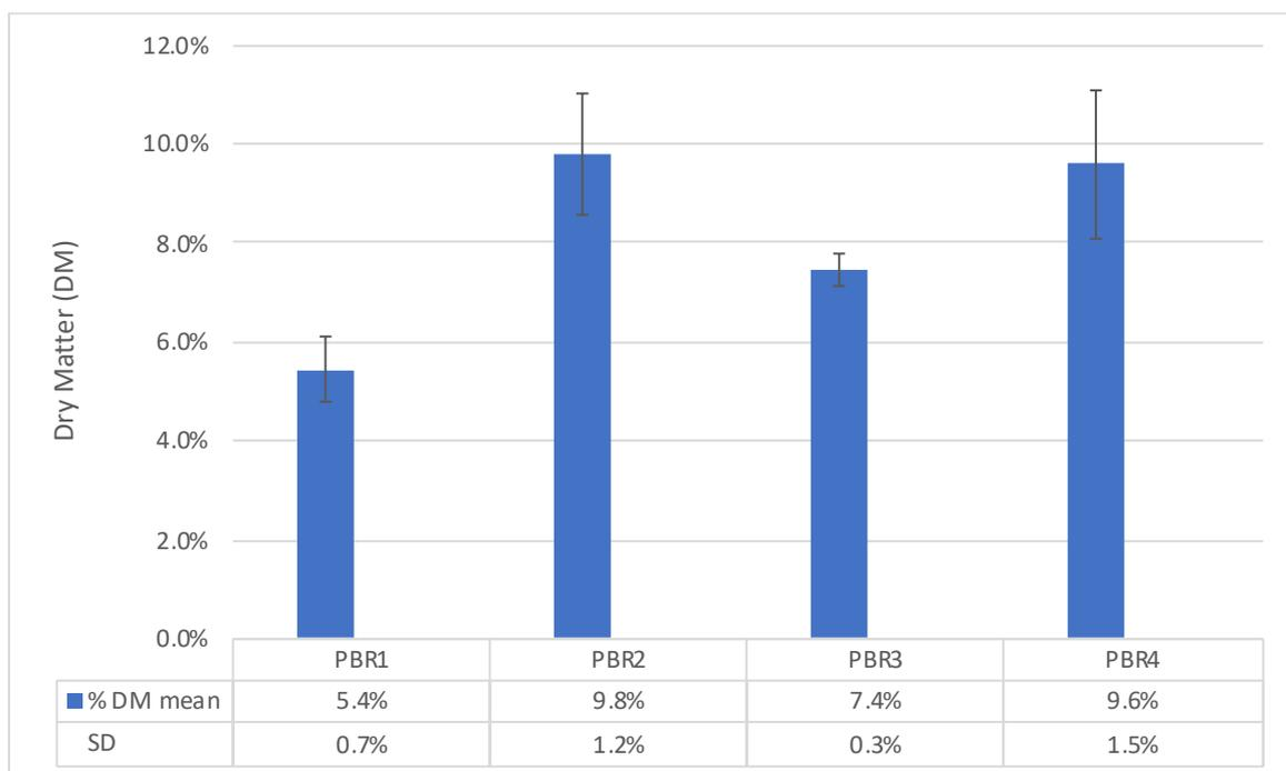
Figure 35 - The bar graph presents a comparison of DM among the four PBRs (PBR1, PBR2, PBR3, and PBR4). Each bar represents the mean DM value for a specific PBR, while the error bars depict the standard deviations.
