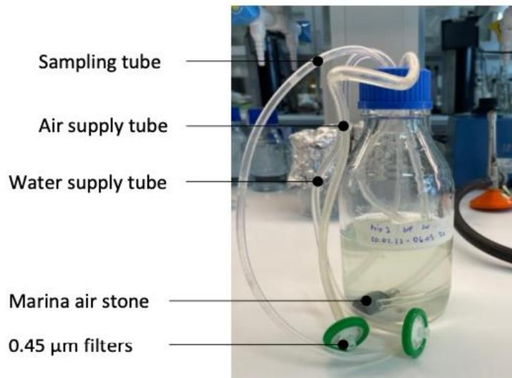
Figure 21 – Picture of the 500 mL blue cap flask used in the experiment. The flask contains a water supply tube, an air supply tube with an air stone for aeration, both tubes are fitted with 0.45 µm filters to prevent contamination, and a sampling tube for collecting microalgae samples.
