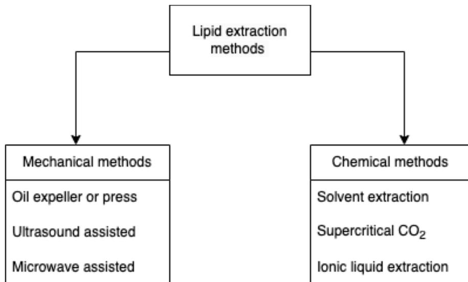
Figure 11- Diagram illustrating different techniques for extracting lipids from microalgae adapted from [126].
