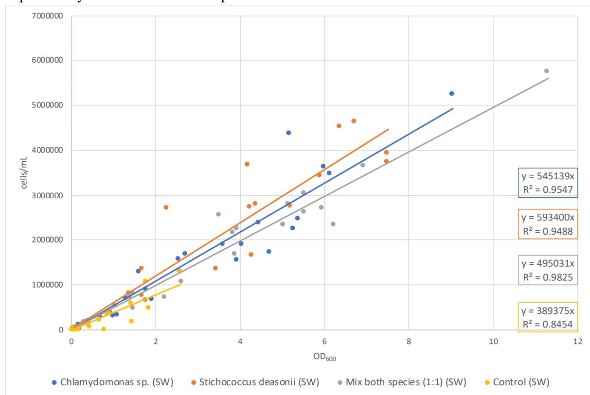
Figure 42- Relationship between optical density (OD<sub>600</sub>) and cell density (cells/mL) in four microalgae cultures grown in artificial saltwater and commercial nutrients medium. Linear trendlines were fitted and the corresponding trendline equations and correlation coefficient (R<sup>2</sup>) was displayed.
