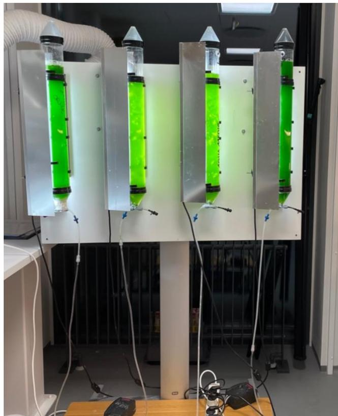
Figure 16 - Picture of 2L photobioreactors containing samples collected at the Esbjerg harbour.
