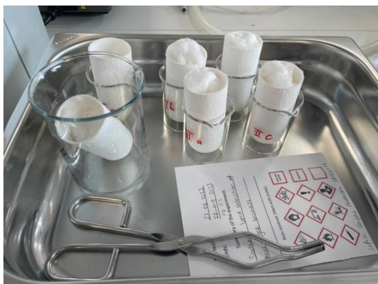
Figure 28 – Picture of thimbles inside labelled beakers and tongs.
