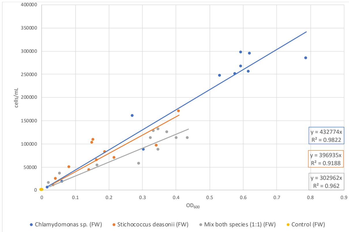
Figure 43 - Relationship between optical density (OD<sub>600</sub>) and cell density (cells/mL) in four microalgae cultures grown in fishwater medium. Linear trendlines were fitted and the corresponding trendline equations and correlation coefficient (R<sup>2</sup>) was displayed.
