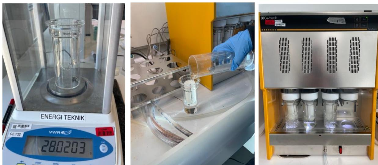
Figure 29 – From left to right: Picture 1: weighing of the soxtherm cup, with the thimble holder and the 3-5 small stones. Picture 2: hexane being poured into the soxtherm cup. Picture 3: Soxtherm.
