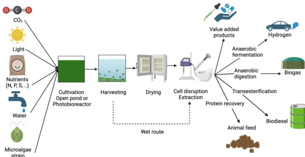
Figure 1 - A simplified pipeline model for a microalgae biorefinery. Created with BioRender.com.
