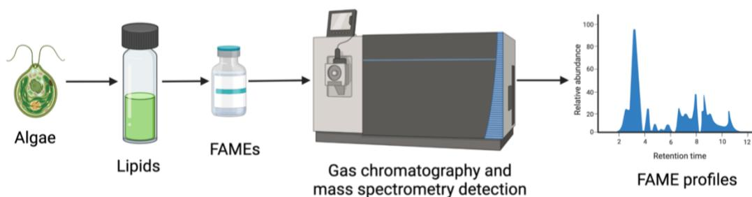
Figure 17 - Schematic representation of the analysis of fatty acid methyl ester (FAME) of microalgae by gas chromatography and mass spectroscopy (GC-MS).
