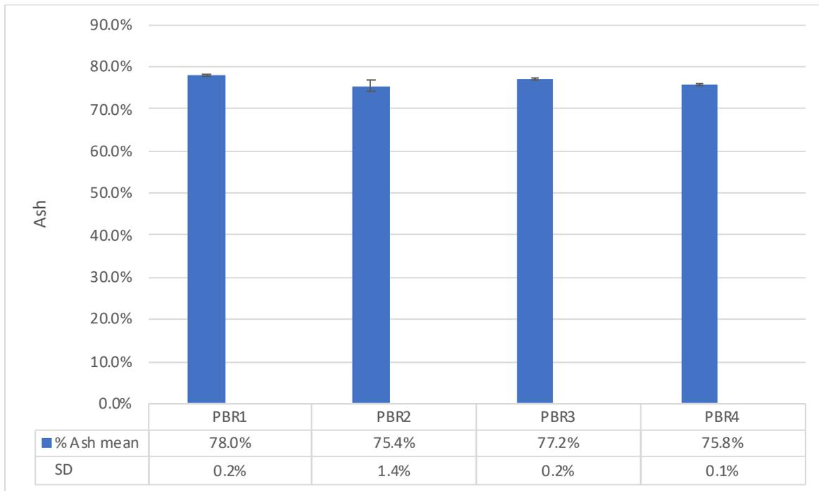
Figure 36 - The bar graph presents a comparison of the Ash content among the four PBRs (PBR1, PBR2, PBR3, and PBR4). Each bar represents the mean Ash value for a specific PBR, while the error bars depict the standard deviations.
