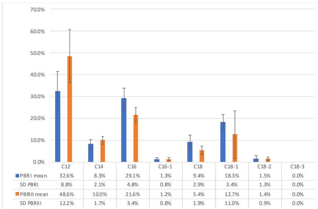
Figure 38 - Bar graph illustrating the relative proportions of different fatty acids in the microalgae oil obtained from PBR1 and PBR3.
