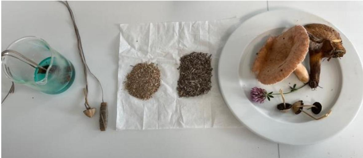
Figure 27- Materials to test any assisted flocculation. From left to right: A thread wrapped around a cardboard and dipped in fertiliser. A small whole mushroom dipped in fertiliser. A small whole mushroom. A thread wrapped around a cardboard. Fine cut fibbers (3g). Roughly cut fibbers (4g). A big white mushroom that will be chopped up (5g). A flower.
