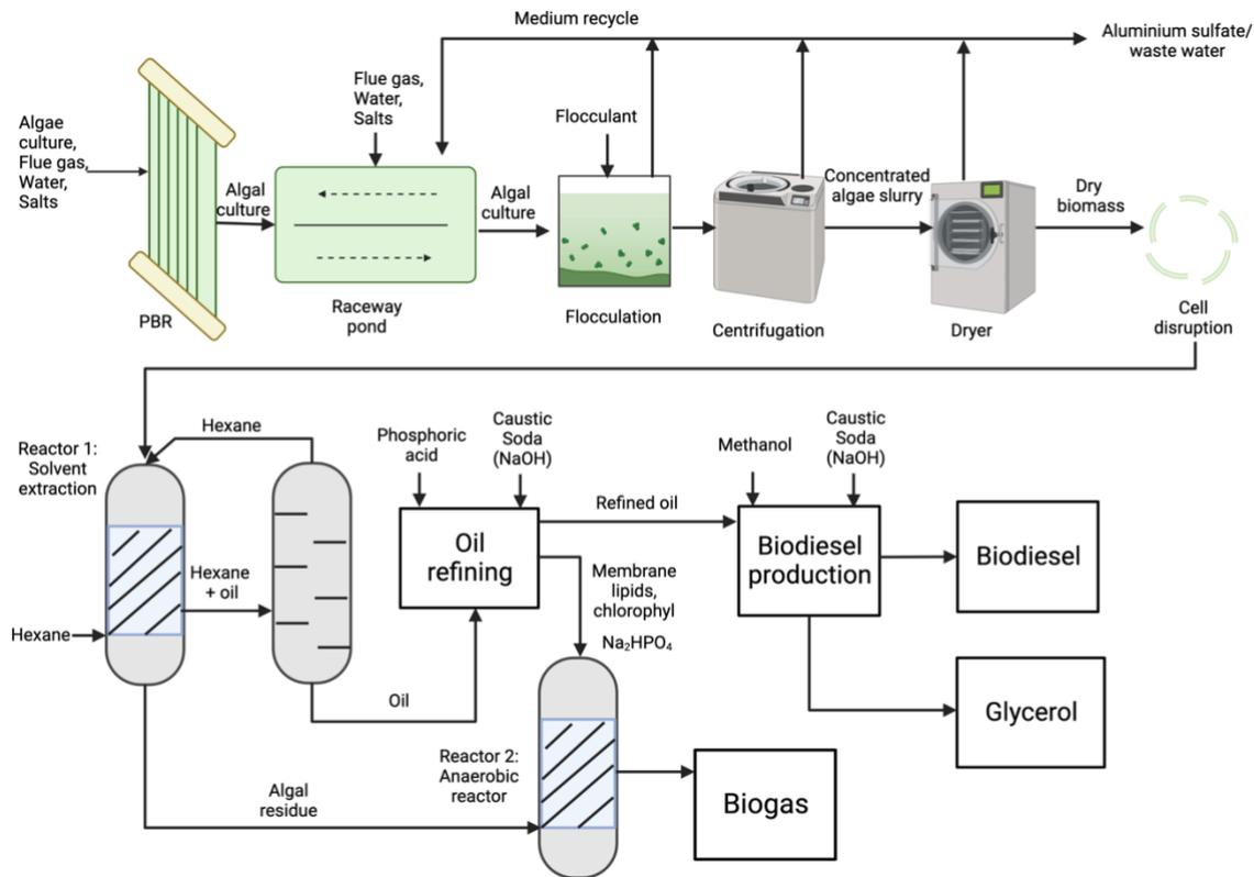
Figure 15- Process flow diagram of a hybrid cultivation system and the downstream processes for the production of biodiesel. This figure was adapted from the study conducted by Adesanya et al. 2014 [138] and Created with BioRender.com.
