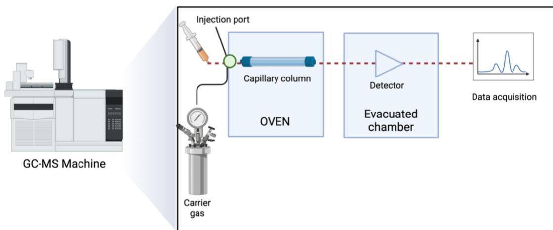
Figure 32 - Schematic representation of a GC-MS apparatus. Created with BioRender.com
