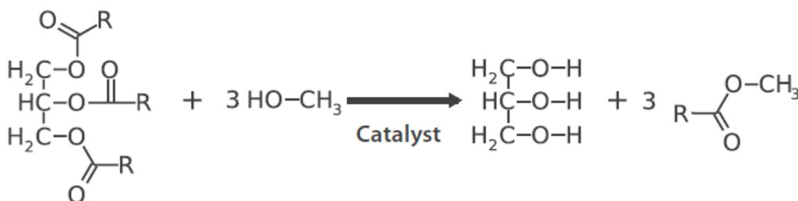
Figure 30 - Fatty acid methyl esters (FAME) reaction. Glycerol-bound fatty acids react with methanol in the presence of a catalyst to give mixture of glycerol and biodiesel (FAME).
