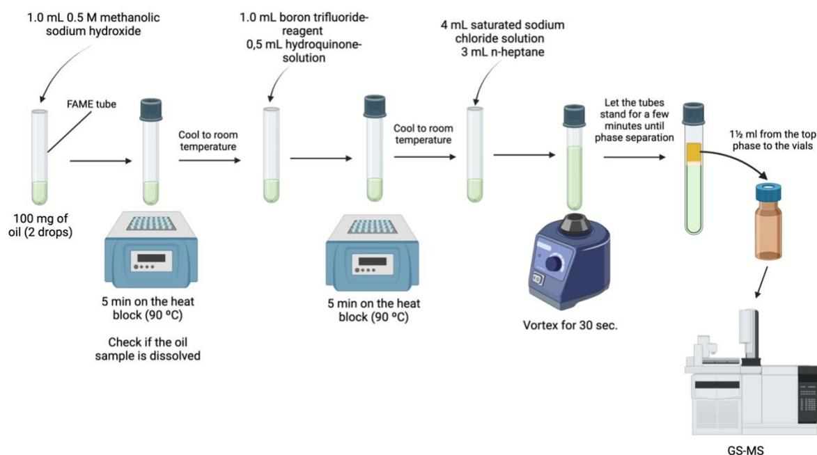
Figure 31-Schematic Representation of the FAME Protocol. Created with BioRender.com.
