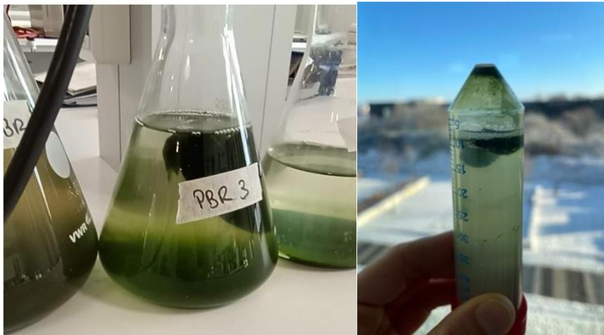
Figure 47 - An atypical aggregation observed in microalgae samples from the 2L photobioreactors left on the counter.
