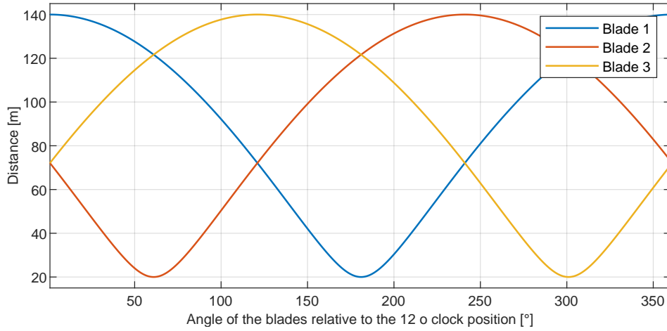
Figure 4.14: Illustration of ADM, based on straight line distance at observer position [0, 0, 0]
