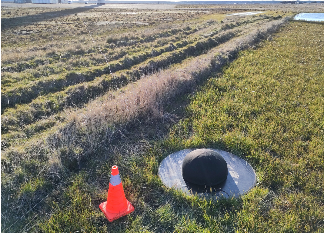
Figure A.4.6: Microphone 200 m in front of the wind turbine (Cyan mic position '3', on fig. A.4.1).
