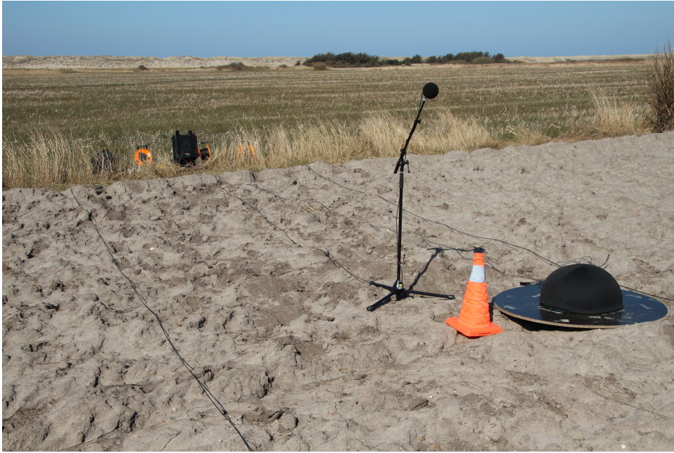
Figure A.4.2: Microphone setup at 400 m.
