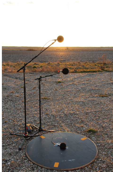
Figure A.4.8: Third microphone setup, with 3 microphones (without secondary windshield).
