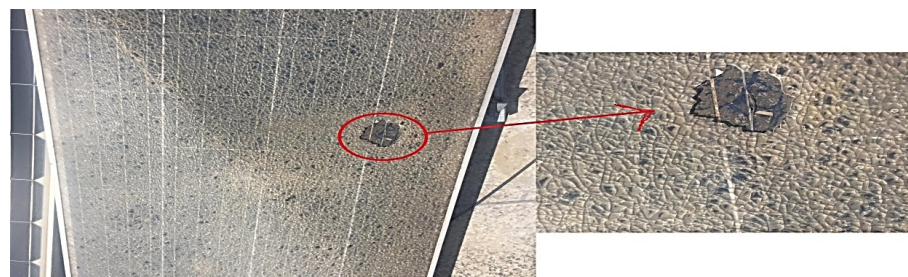
Figure 2. Glass protection breakdown-PV module Located in Islamabad, Pakistan.
