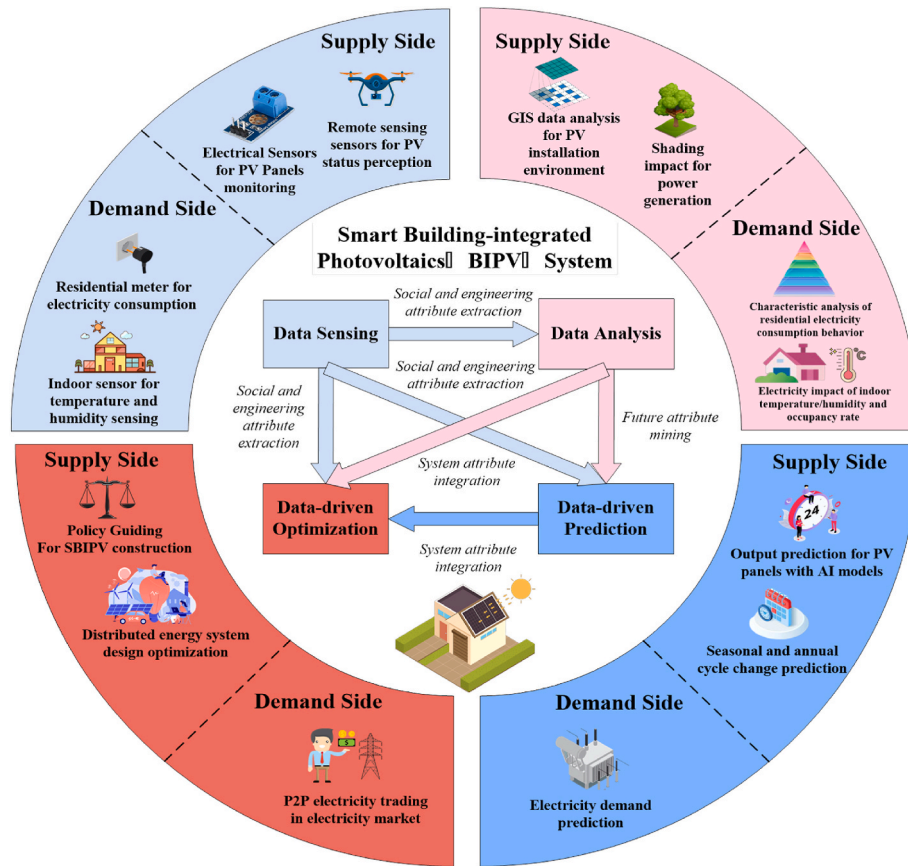
Fig. 1. Structure diagram of data-driven SBIPV systems.
