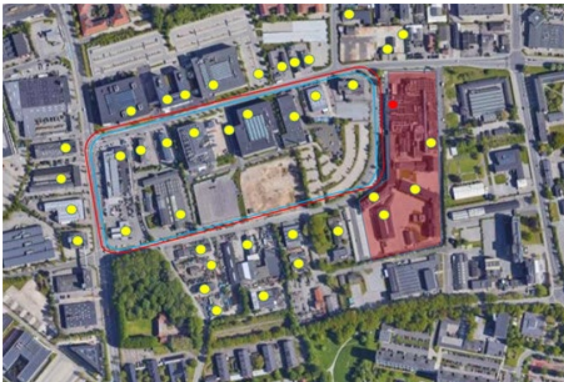
Figure 7: Commercial area in northern Copenhagen – the red point represents the excess heat available, while the yellow ones the consumers for the specific area
