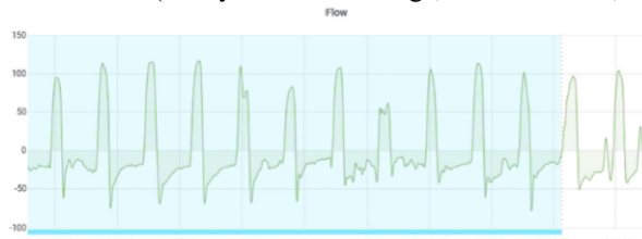
Figure 2. Excerpt of the flow graph of the annotated ventilation data in Grafana
