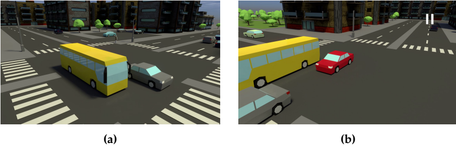
Fig. C.3: An illustration of the output from a camera mounted in existing infrastructure is seen in (a). Given this view-angle, the bus and other large objects clearly introduce an occlusion problem as illustrated in (b).
