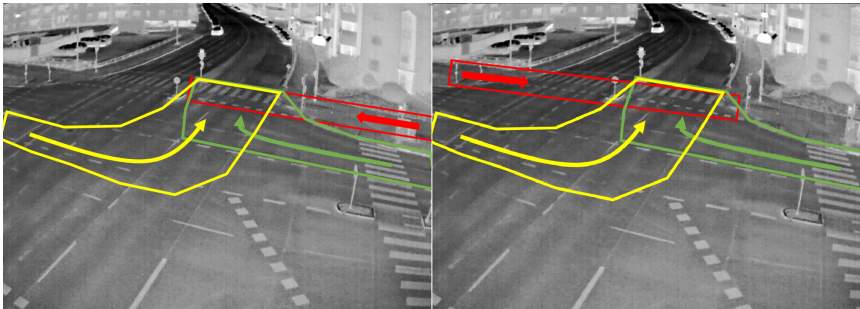
Fig. J.7: The goal is to find times when a vulnerable road user is moving through the red regions in the marked directions, while a car is moving either through the green or yellow regions simultaneously.
