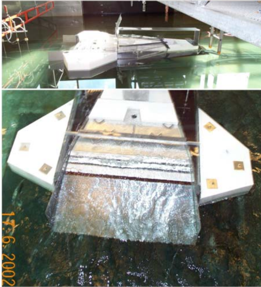
Figure 4.22: Photos of the floating model of the Power Pyramid in calm water (top) and in action in irregular waves (bottom).
