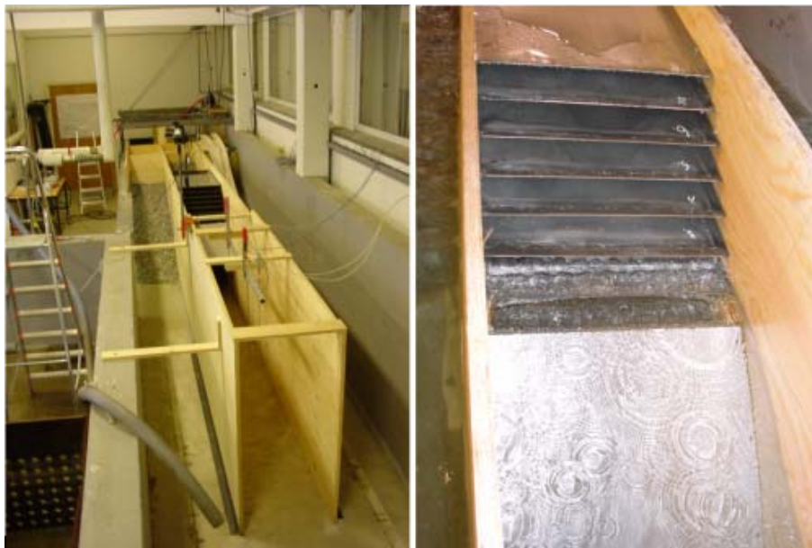
Figure 4.5: Drawings and photos of the model test setup as constructed in the wave flume. Top: Plan view. Middle: Cross section A - A and B - B. Measures are in mm (model scale). Bottom, left: Model test setup before the flume is filled with water. Bottom, right: The model in action.
