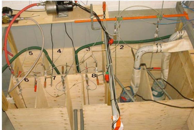
Figure 4.6: Tanks used for measuring overtopping of the 8 reservoirs with pumps and level gauges mounted.
