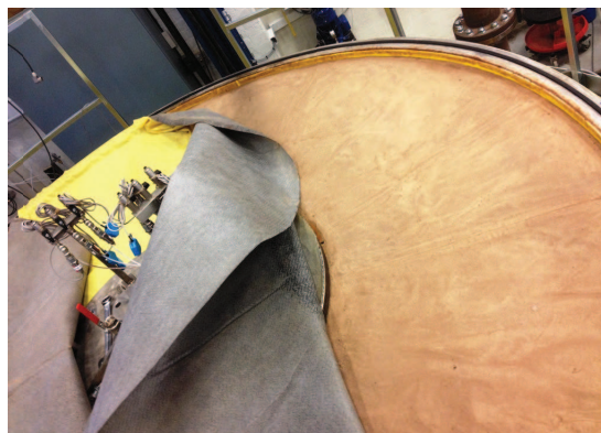
Figure 4.12 Slightly moist sand after a test with the membrane pressure.
