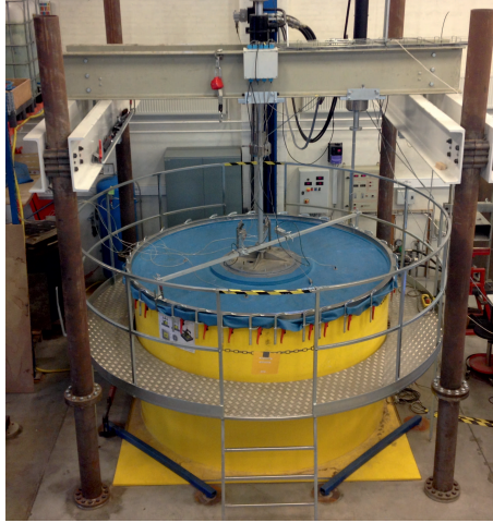
Figure D.3 Test set-up for the axial bucket foundation testing with applied overburden pressure.
