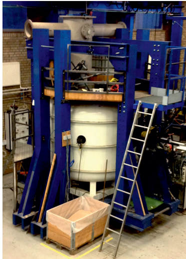
Figure 4.17 Pressure tank used for the displacement rate tests.
