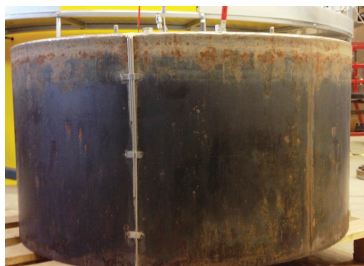
Figure 4.10 Bucket foundation model, 1 m in diameter and 0.5 m in skirt length.
