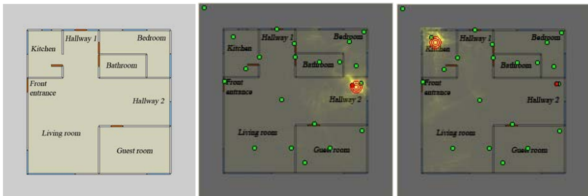
Figure 6.10 Resident's home (left), probability maps and calculated positions for the resident (middle) and for tracked medication (right)
