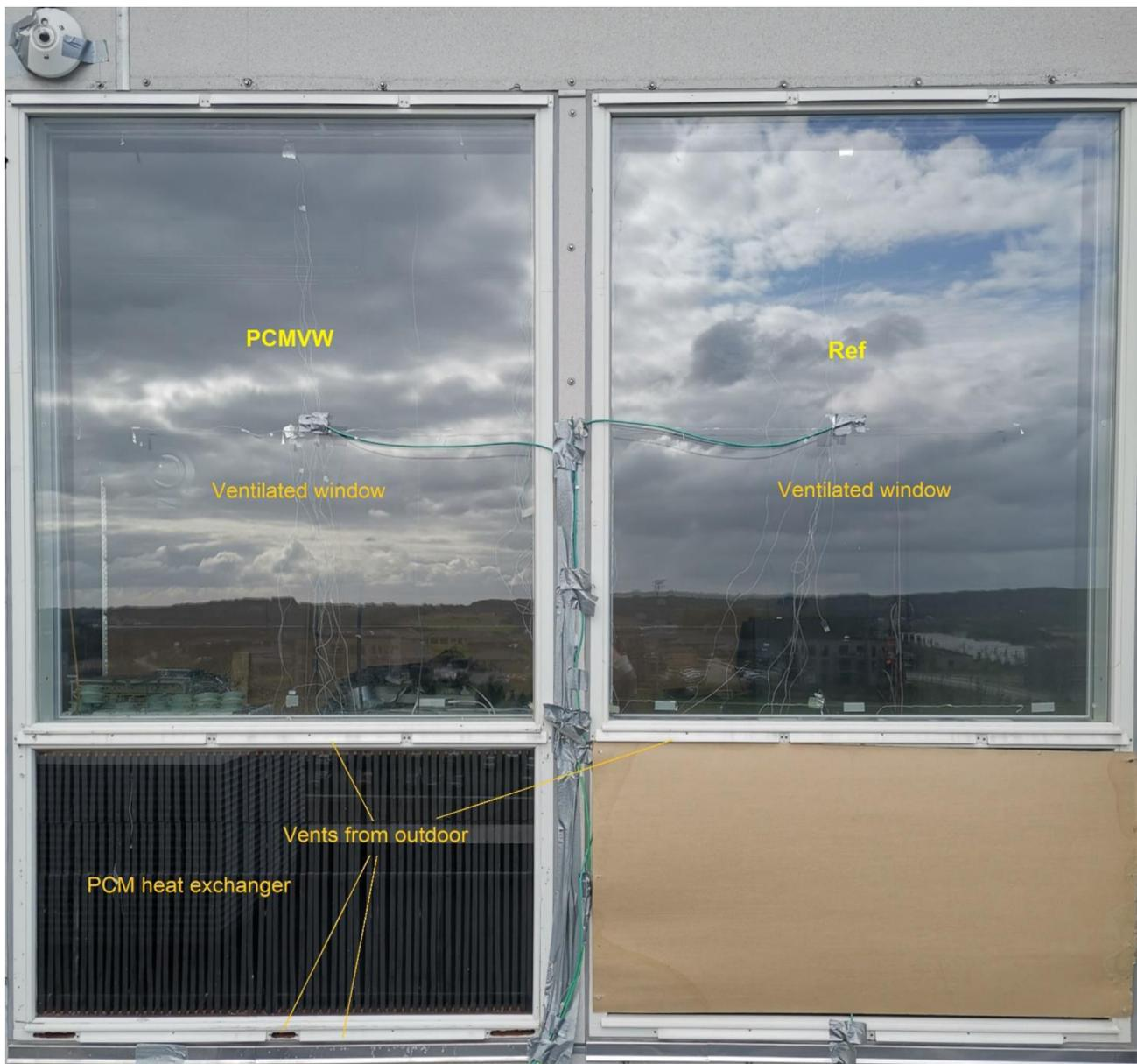
Fig. 1. Experimental setup. The PCMVW in the left and the Reference window in the right.
