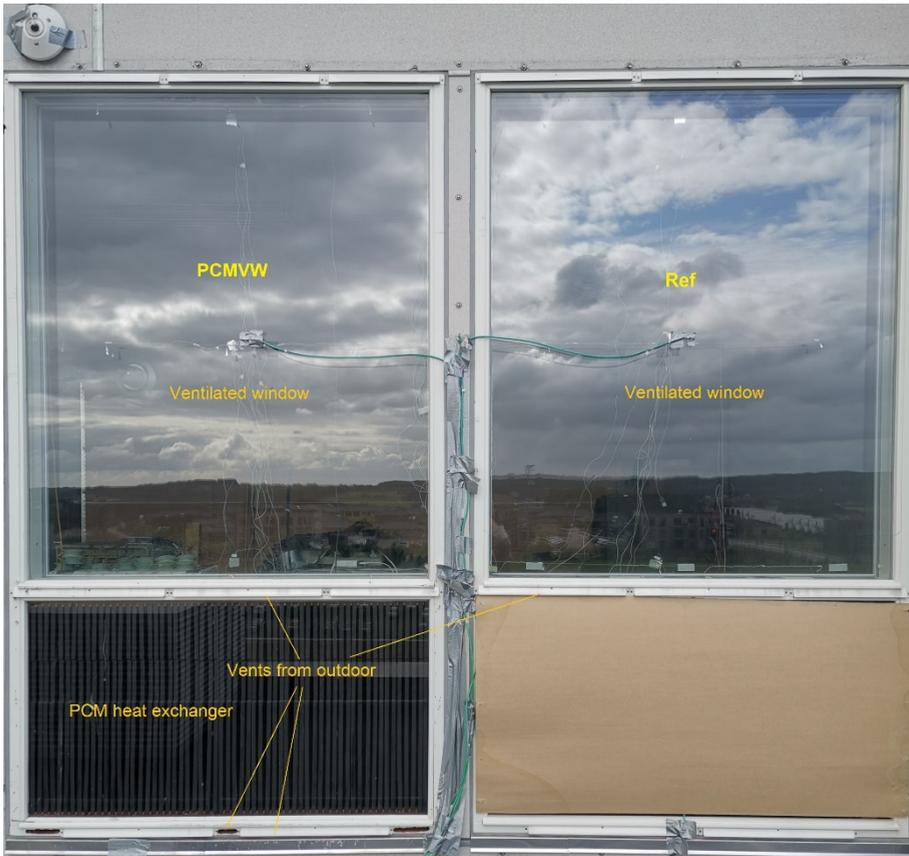
*Figure 4-1 The experimental setup of PCM-VW and reference VW.[27]*
