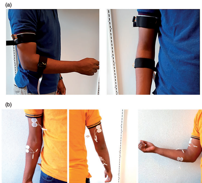
Figure 2. Sensor placements on human arm, (a) FMG and (b) sEMG.
