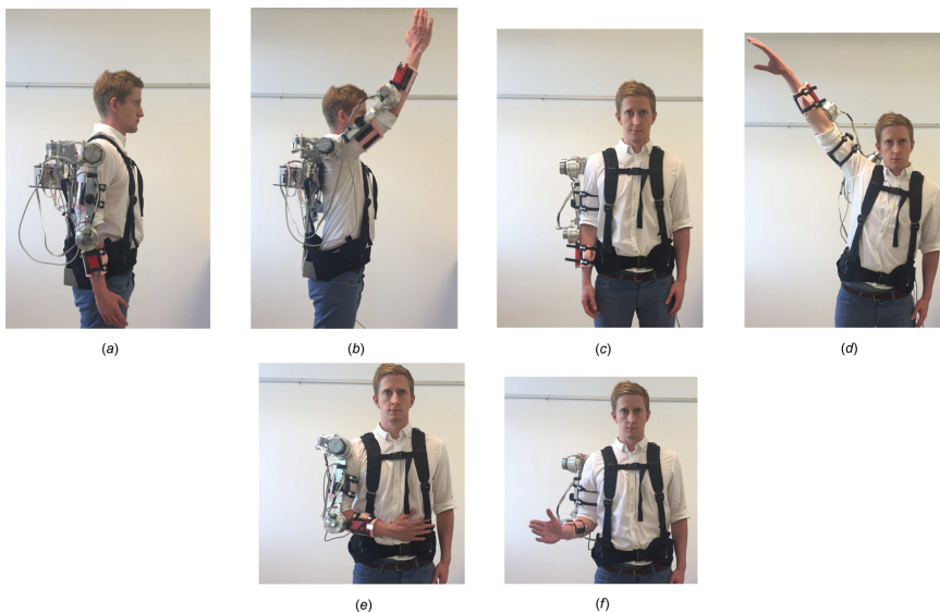
Fig. 12 The shoulder joint mechanism in the AAU exoskeleton in (a) 0 deg shoulder extension, (b) 170 deg shoulder flexion, (c) 0 deg shoulder adduction, (d) 120 deg shoulder abduction, (e) 90 deg shoulder internal rotation, and (f) 20 deg shoulder external rotation
