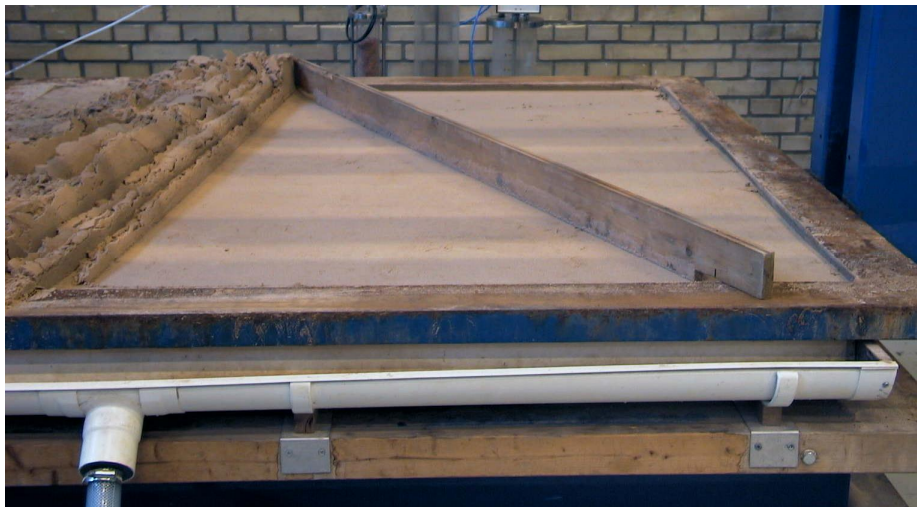
Figure 2.26 Alignment of the soil surface after preparation.
