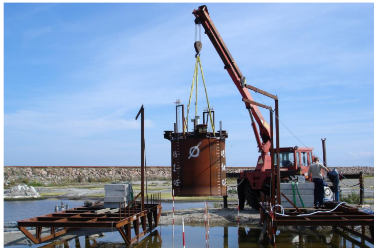
Figure 3.2 Bucket foundation used in large scale tests.
