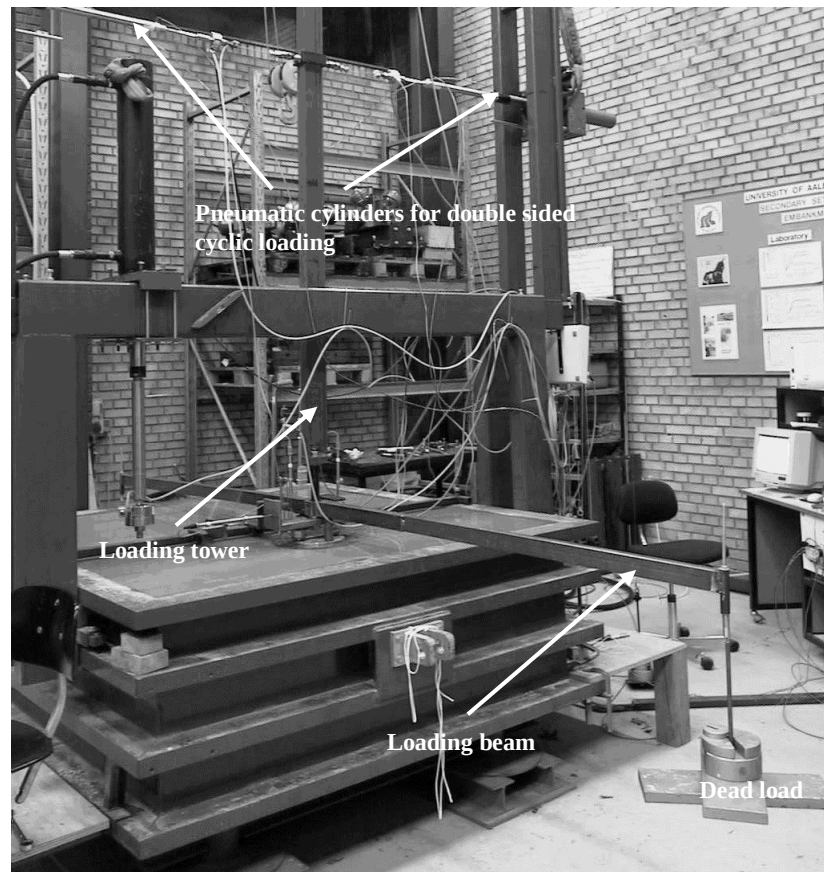
Figure 2.33 Excess vertical load applied by use of loading beam.
