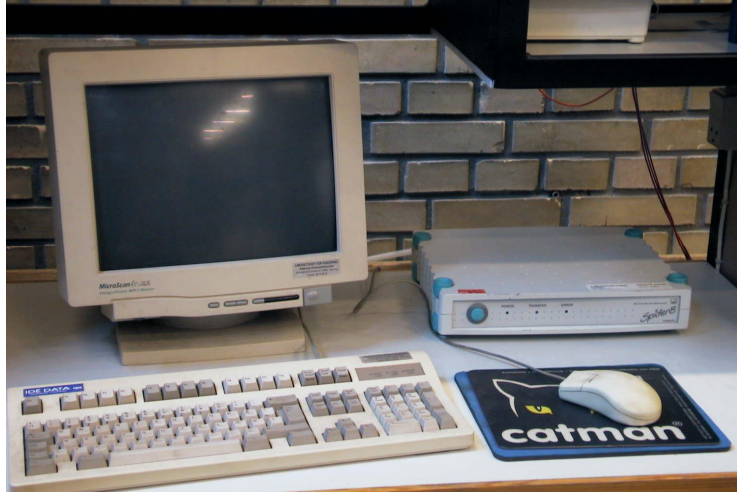
Figure 2.22 Spider 8 Sampling device connected to a PC.
