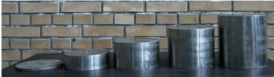
Figure 2.1 Bucket foundation tested in the laboratory. D=200\text{mm} and d/D=0; 0.25; 0.5; 0.75 and 1 are shown.
