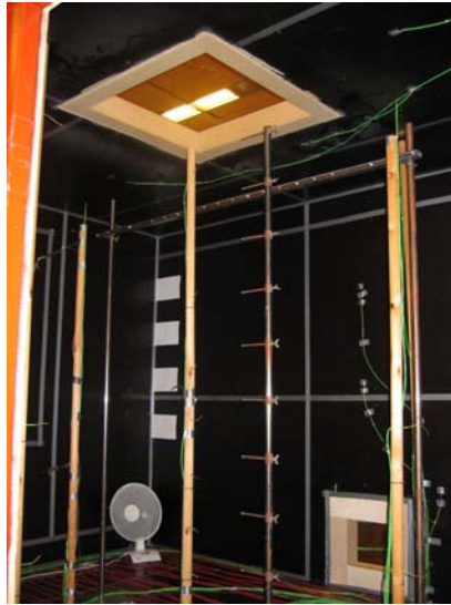
Figure 3.9: The inside view of the test room. The side length of top horizontal opening S_T=0.8\text{m} , the side length of bottom vertical opening S_B=0.3\text{m} , and the opening ratio A_T/A_B=7.11 .
