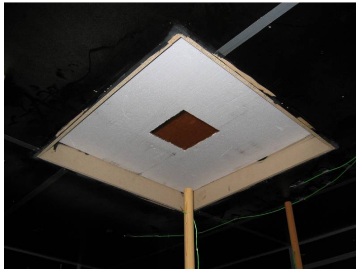
Figure 3.8(A): The metal plate with opening from inside view of the test room.
