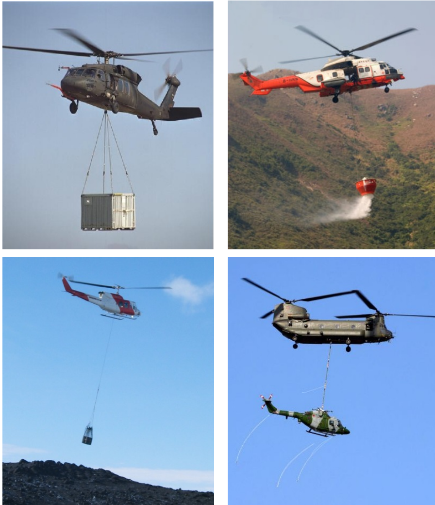
Figure 1.1: Top left: UH-60 Black Hawk with a container load. Top right: Eurocopter Super Puma used for fire fighting. Bottom left: Bell 212 with slung load. Bottom right: CH-47 Chinook towing a Lynx fuselage.
