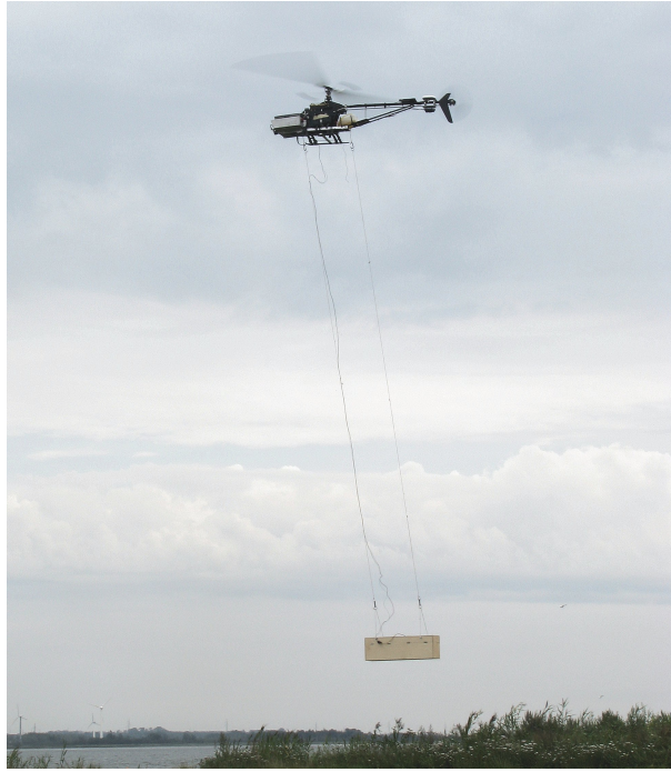
Figure 2.6: The AAU Bergen Industrial Twin flying with the dual wire demonstration slung load.
