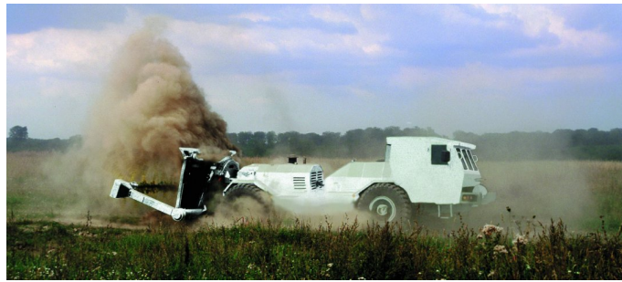
Figure 1.5: The demining flail truck build by Hydrema.
