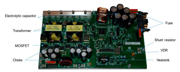
Figure 2. Critical power stage subcomponents in a power conditioner used in PEMFC.
