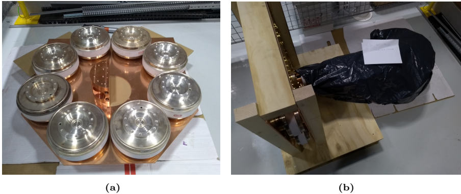
Fig. 2.6: Photographs of the resonant tank, with (a) the capacitor bank with 8 vacuum capacitors in parallel for a total capacitance of 40 nF and (b) the complete resonant tank including proprietary induction coil mounted in a wooden chassis.
