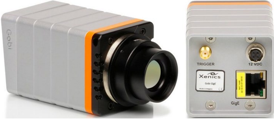
Fig. 2.5: The used thermal camera Xenics Gobi-384-GigE. Image source: © Xenics.
