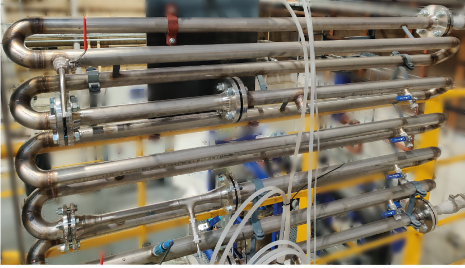
Fig. A.2: In-line pre-treatment static flocculator. The flocculator consists of a set of 180^\circ pipe bends and a metal coagulant is dosed at the inlet of the application and the dosing of the cationic polymer is performed after a total of 4 \times 180^\circ pipe bends. The particle size distribution is measured at the outlet of the static flocculator.
