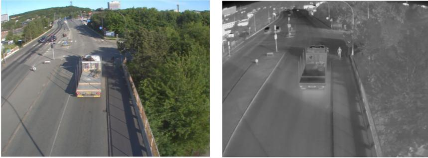
**Fig. J.1:** Shadows complicates the detection of a cyclist in the RGB recordings, whereas the cyclist is easily distinguished from the background in the thermal recording.
