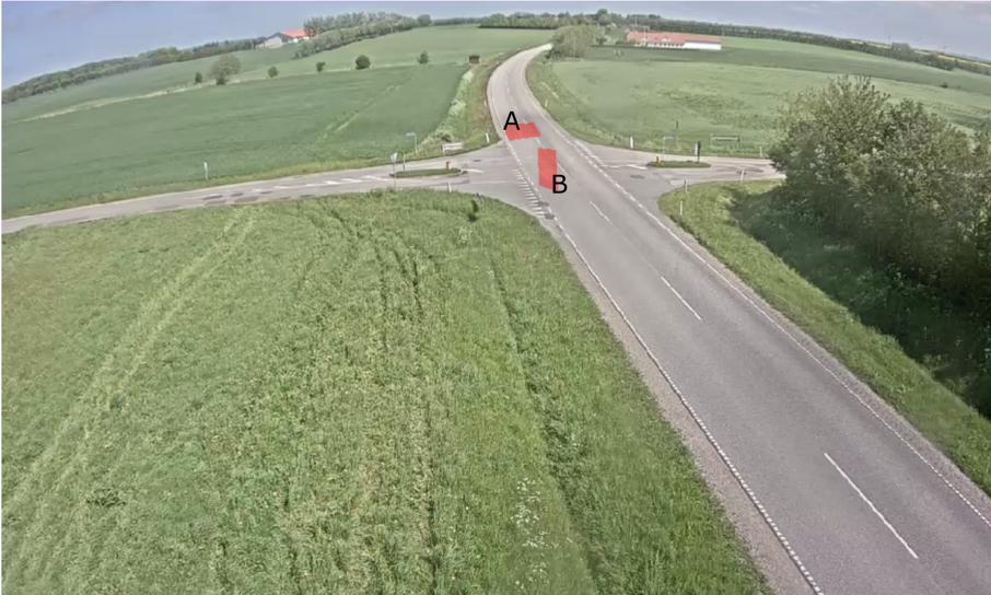
Fig. L.19: Two movement detectors registered the traffic flows through the detectors.
