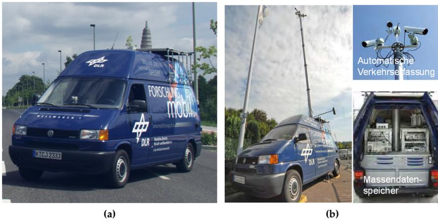
**Fig. L.8:** (a) The DLR UTRaCar with retracted telescopic mast. (b) The DLR UTRaCar with extracted telescopic mast. [9]
