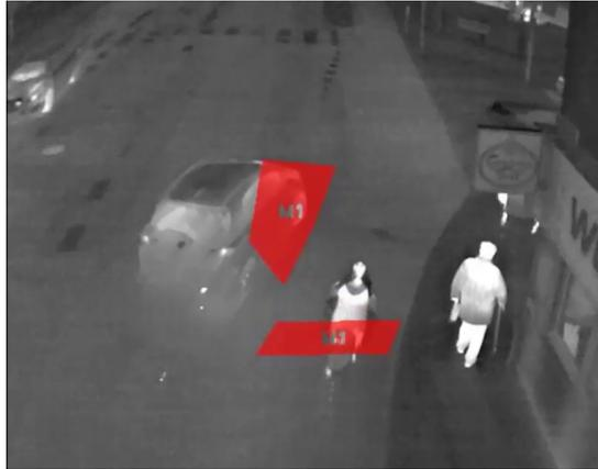
**Fig. 3.5:** A sample use-case of the RUBA software. Two detectors are defined to find possible encounters between cyclists and right-turning vehicles.
