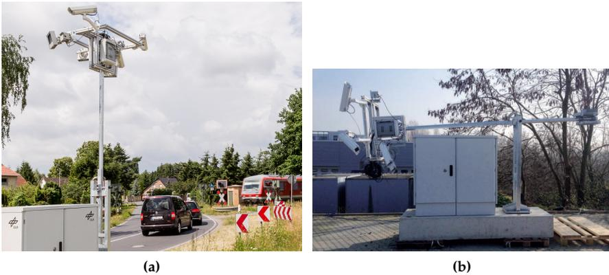
Fig. L.11: (a) DLR Setup in operation mode. (b) DLR Setup in transportation mode. [17]
