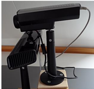
**Fig. B.2:** Camera configuration. The RGB and thermal sensor are vertically aligned.
