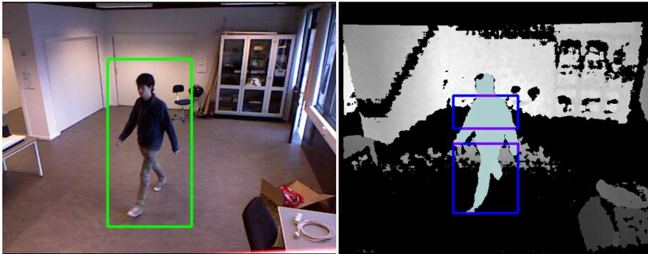
**Fig. C.3:** The left image illustrates a detection. On the right, the person has been segmented in the depth image, and the blue boxes illustrate the boxes which are used as basis for the color histograms.
