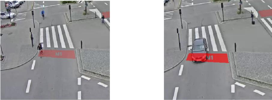
Fig. K.5: Demonstration of the ability to only detect cars, trucks and buses, and not bicycles.
