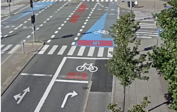
**Fig. K.3:** Double module to detect same time arrival between a straight going bicycle and a right turning car and a straight going bicycle and a left turning car.
