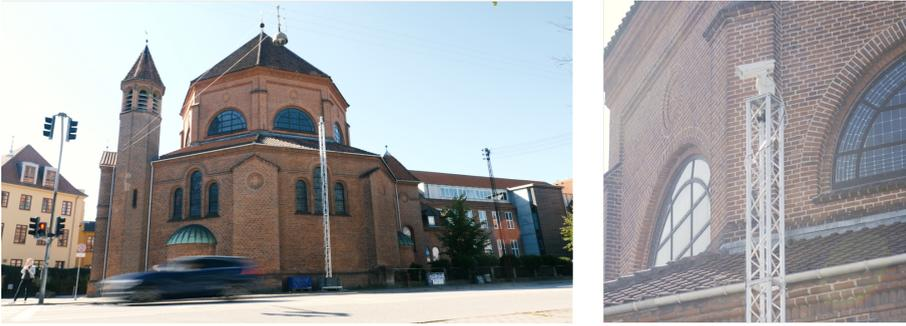
**Fig. L.15:** The portable pole deployed at traffic intersection. The pan-tilt motor with one RGB camera is installed on the top of the pole, which makes the RGB camera adjustable remotely.
