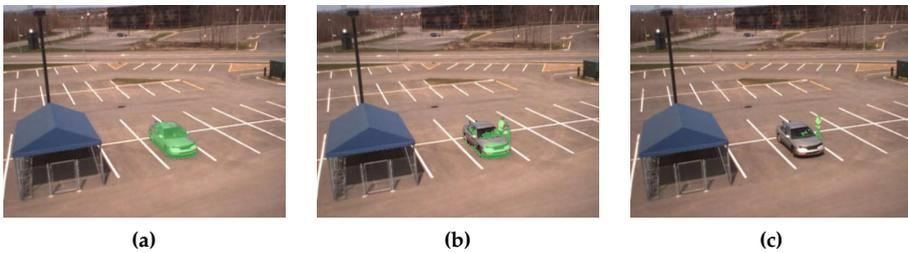
Fig. E.17: The parked car gradually merges into the background by using a standard GMM segmentation method (foreground marked green). (a) Car arrives; (b) Car has stopped for several frames; (c) Driver got out the car. The proposed method mitigates this issue by predicting foreground regions and lowers the update rate  $\alpha$  correspondingly. From [2].
