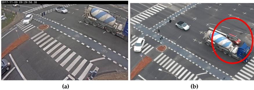
**Fig. L.1:** Objects can overlap each other in the camera-view as seen in (a) where the the large cement truck clearly occludes the lane behind it. (b) clearly shows that a red car is in fact driving side-by-side of the cement truck.
