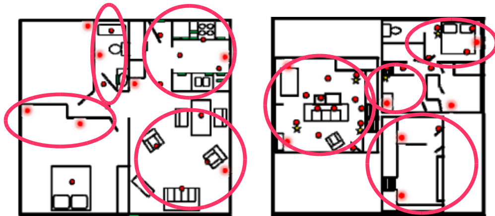
Figure 7.14. Bosch and Cairo test-bed smart environments used by Cook (2012). The encircled sensor groups are the opportunities for sensor cluster-tree grouping. The small red dots are the smart home sensors.
