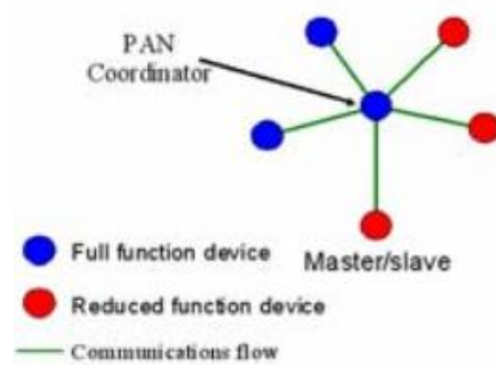
Figure 7.15. ZigBee cluster-tree topology (Kim et al., 2008) .
