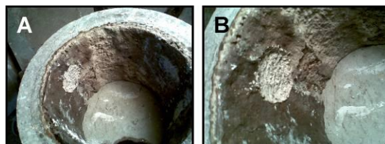
Figure 4.8. Photos of a concrete pipe segment after sampling. The sampling area is seen as the light area in the corrosion products (Jensen et al. , subm. (VI)).
