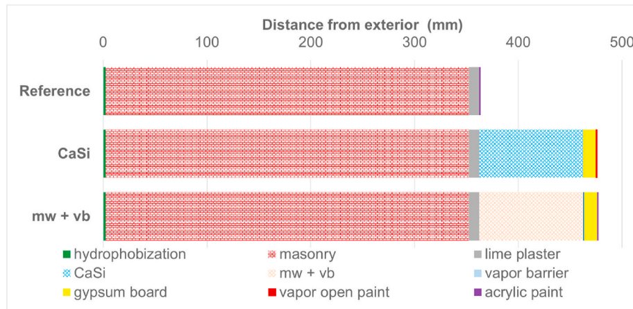
Fig. 2. Wall configuration without (reference) and with internal insulation. Hydrophobization: 2.4 mm impregnation depth, masonry (Y brick): 350 mm, lime mortar: 10 mm, insulation system: 100 mm, gypsum board: 12.5 mm, vapor open paint sd = 0.01 m, vapor barrier (vb) sd = 70 mm (mineral wool (mw) system) and acrylic paint sd = 0.18 m. sd: equivalent air layer thickness ( \mu \cdot material thickness).
