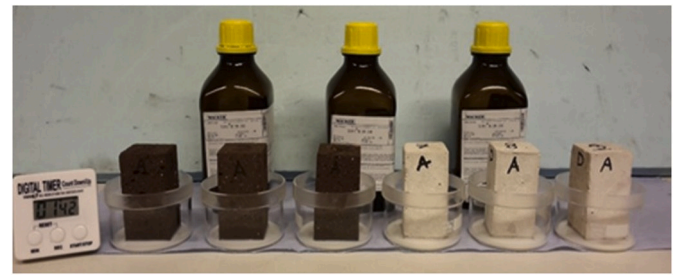
Fig. 3. Impregnation of brick (left) and mortar (right) samples by exposing them to free uptake of water repellent agent (liquid products).
