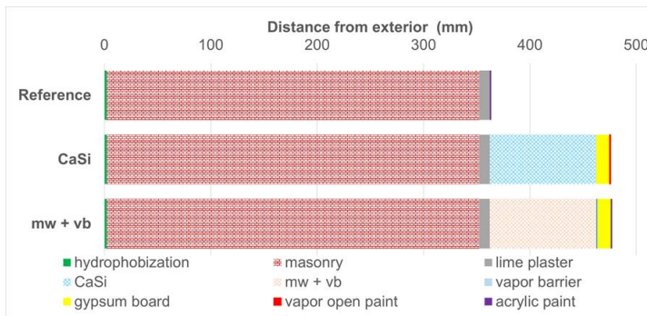
Figure 3- 2 Wall configuration without (reference) and with internal insulation. Hydrophobization: 2.4 mm impregnation depth, masonry (Y brick): 350 mm, lime mortar: 10 mm, insulation system: 100 mm (mineral wool or CaSi), gypsum board: 12.5 mm, vapor open paint with sd = 0.01 m, vapor barrier (vb) sd = 70 m (only for the mineral wool (mw) system) and acrylic paint sd = 0.18 m. sd : equivalent air layer thickness ( \mu \cdot material thickness) (Paper III).
