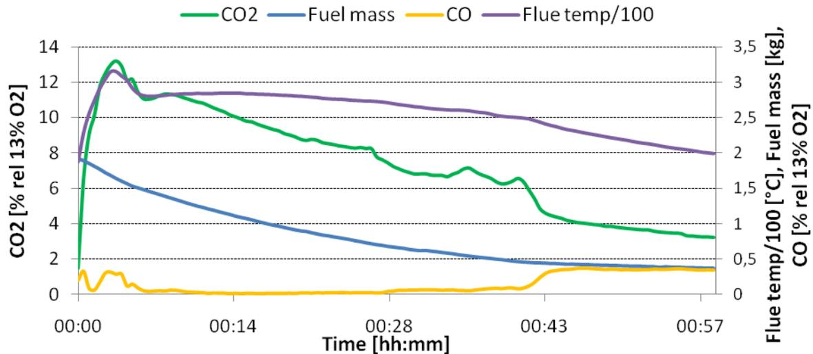
Figure 2. Fuel consumption, CO and CO<sub>2</sub> concentration (13% O<sub>2</sub>, dry gases) in the flue gas and temperature of the flue gas over the test period in the Danish stove.
