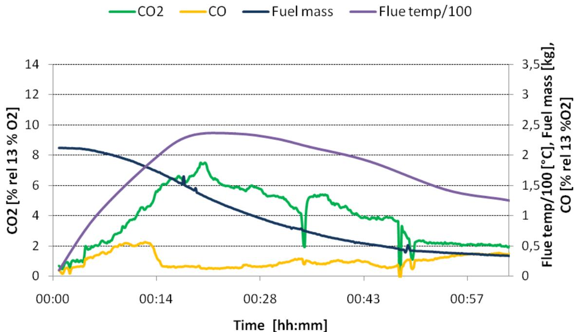
Figure 1. Fuel consumption, CO and CO<sub>2</sub> concentration (13% O<sub>2</sub>, dry gases) in the exit flue gas, and temperature of the flue gas over the test period in the Portuguese stove.
