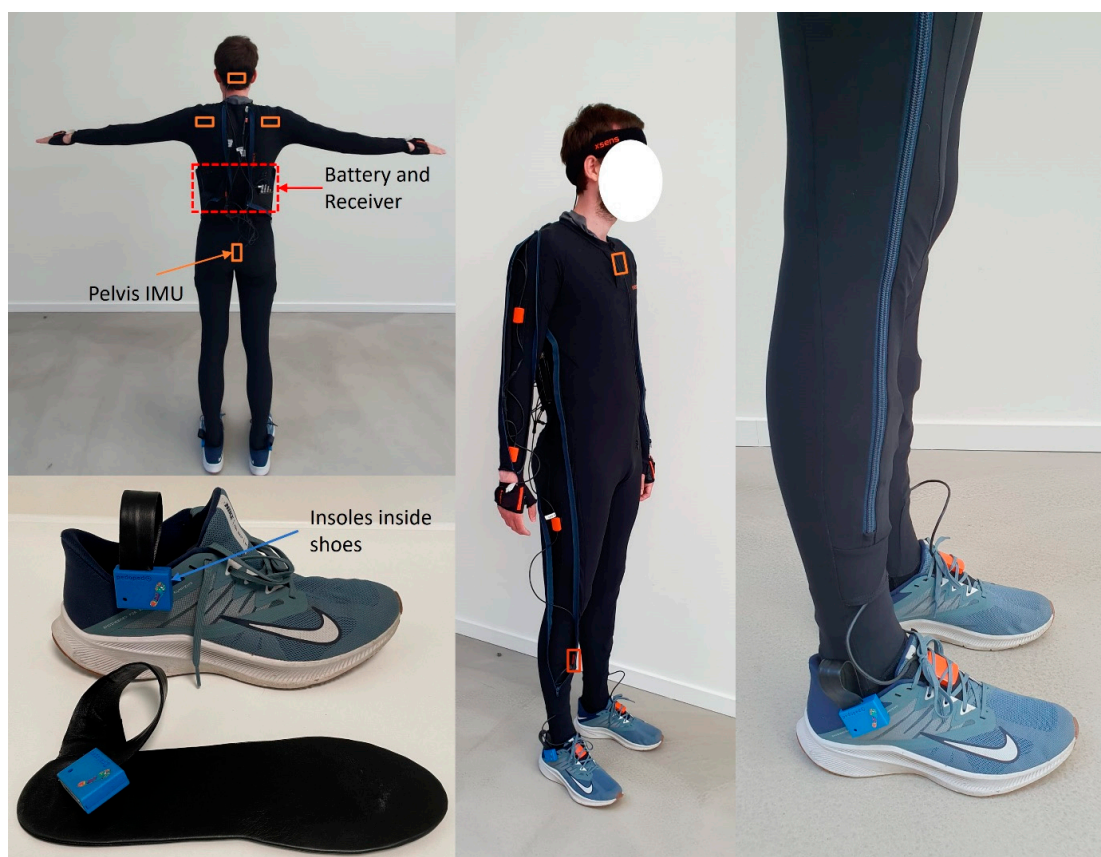
Figure 1. Instrumentation of the 17 IMU sensors (orange boxes), battery, receiver, and shoe insoles. Please note that IMUs were placed on the interior of the suit and symmetrical between the limbs but the suit is unzipped for visualisation purposes.
