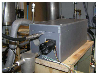
Figure 1: Left: Schematic of the fuel cell system. Right: Picture showing a HTPEM stack prototype.
