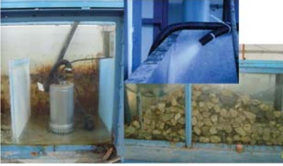
Fig.5. The recirculation system
