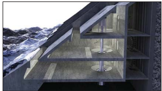
Fig.1. Artistic representation of one 3-level SSG with multistage turbine.
