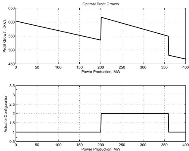
Fig. 2. Optimal growth of profit and actuator configuration.
