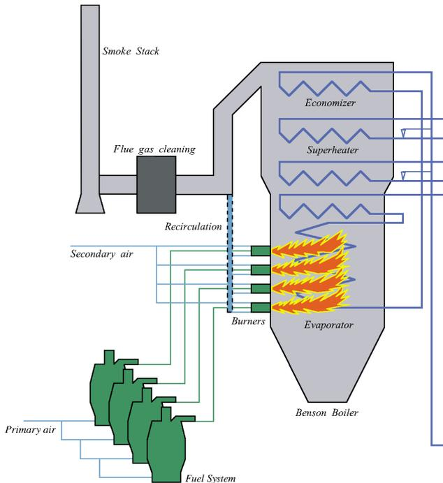
Fig. 1. Scheme of the Benson boiler model.
