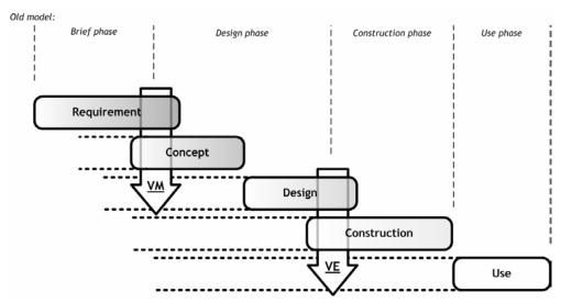
Figure 4.2. The phases of building project illustrating where VM and VE should be applied. It is worth notifying that the time dimension of the figure is out of scale. The figure is made to illustrate the overlap of the phases. At the top the names of the phases in the old model are displayed to illustrate the connection between the old and the new model.
