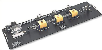
Fig. 8. Experimental version of the ACC benchmark problem
