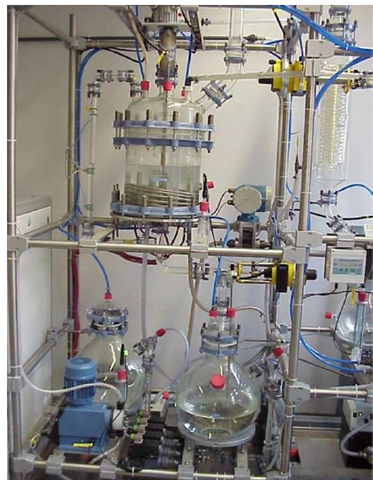
Fig. 1. The experimental pH neutralization plant.
