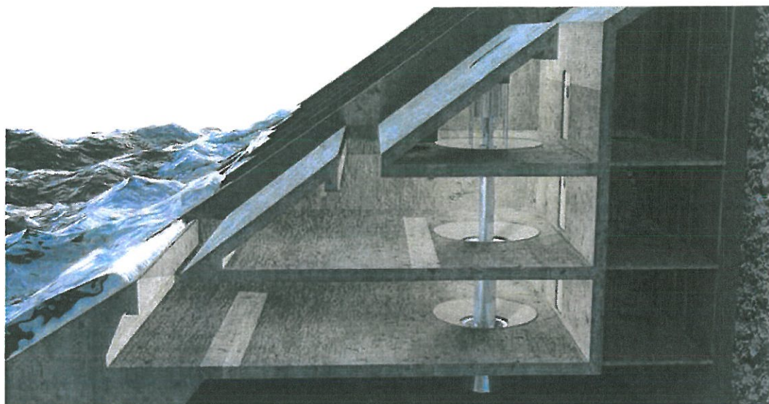
Figure 1. Scheme of Seawave Slot-Cone Generator (SSG).
