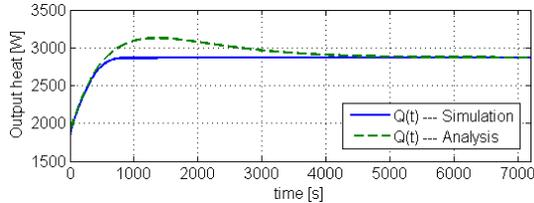
Fig. 6. Simulation and analysis results for  $Q(t)$ . The analytic solution gives us a good enough approximation of the transient and final behavior of the radiator output heat. We utilize this analytic solution to extract the parameters of a first order approximation of  $Q(t)$  step response.
