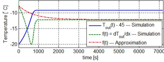
Fig. 5. Simulation results for scaled  $T_{out}(t)$ , its first position derivative and its approximation are shown. The first position derivative i.e.  $f(t)$  is approximated with an exponential function.
