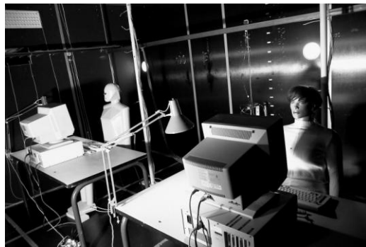
Figure 11. Furnishings and heat load of the IEA Annex 20 room (office layout). The heat load consists of two PCs, two desk lamps and two manikins producing a total heat load of 480 W.
