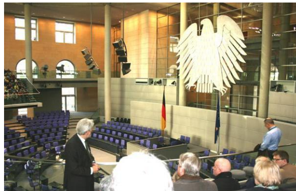
Figure 7. Displacement flow with diffuse floor inlet. a_o/A = 1.0 . The photo shows the Reichstag in Berlin with supply air flow through the carpet.
