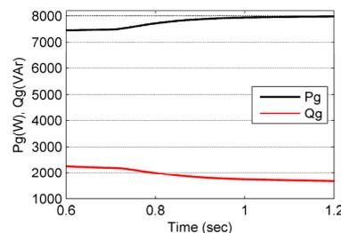
Fig. 7. Utility grid active and reactive powers.
