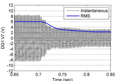
Fig. 10. 5<sup>th</sup> and 7<sup>th</sup> voltage harmonics of DG1
