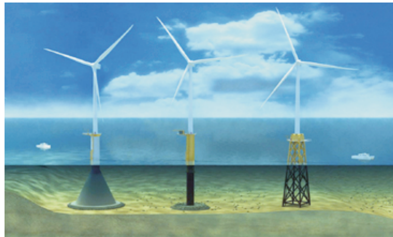
(a) Gravity structure (b) Monopile (c) Jacket
