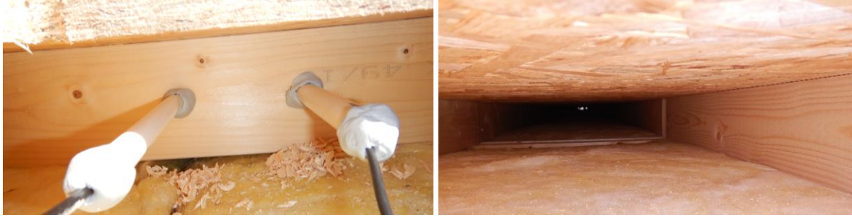
Figure 2. Installation of the measuring devices and overview of the air cavity.
