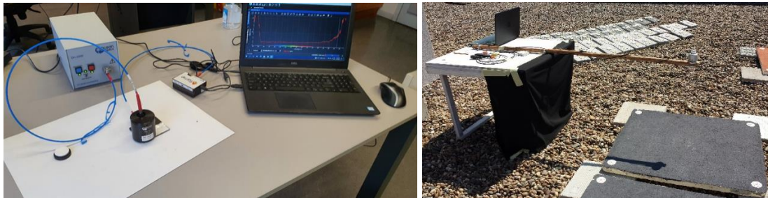
Figure 3. Spectrophotometer and pyranometer measurements.
