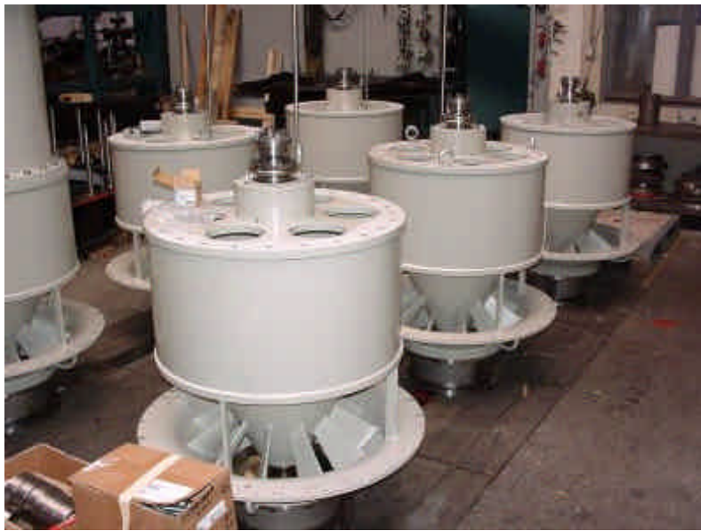
Figure 6: The six axial propeller turbines being assembled at Kössler GmbH (left) and one of the turbines being installed on the prototype in open sea
