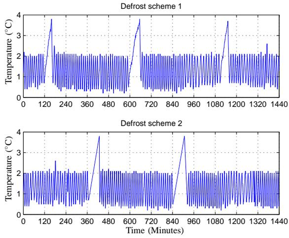
Fig. 6. Air temperature for defrost scheme 1 and 2
