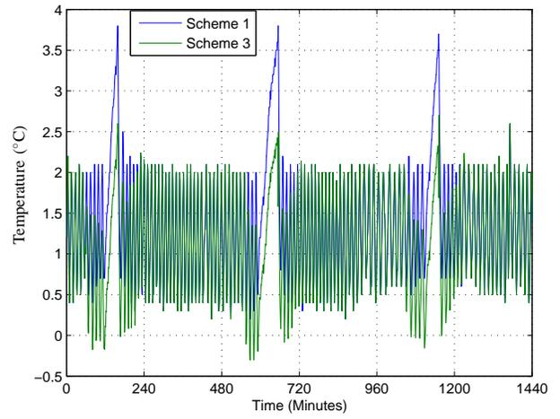
Fig. 9. Air temperature for Defrost scheme 1 and 3
