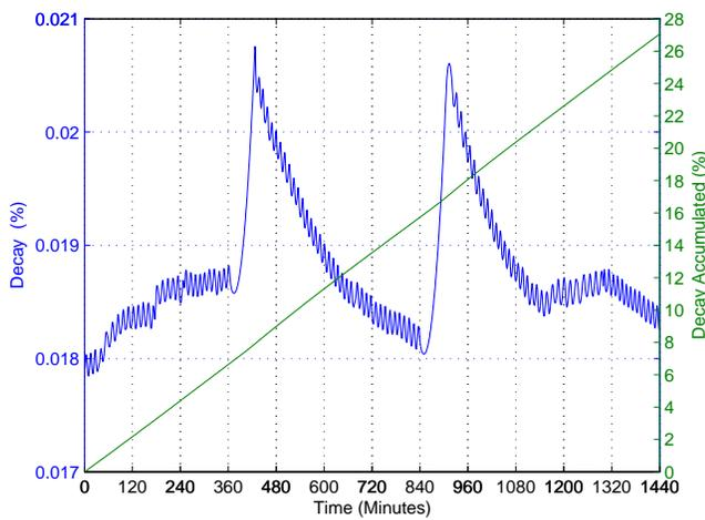
Fig. 8. Fresh fish decay for defrost scheme 2
