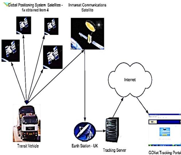
Fig. 4 GCNet Satellite Tracking System
