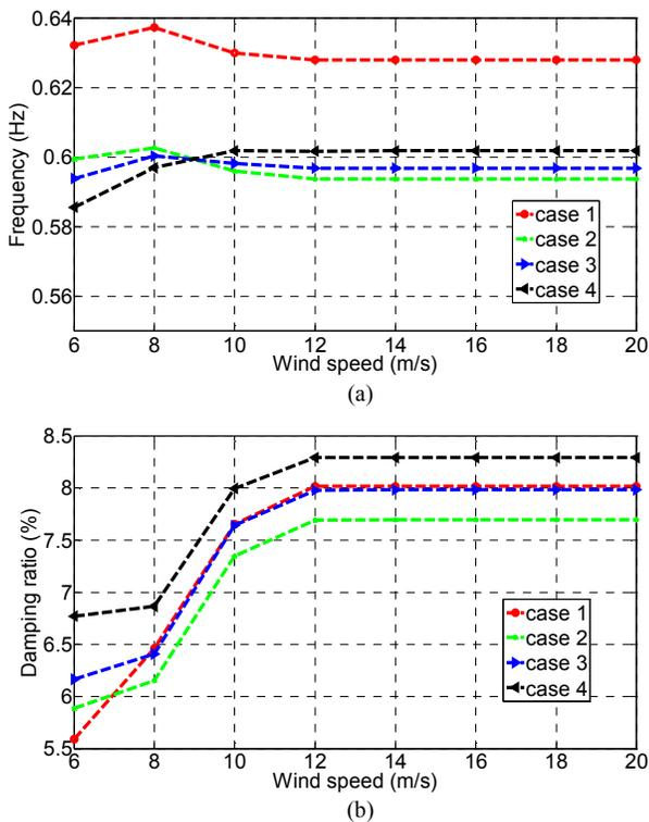
Fig. 7. Influence of wind power ancillary voltage controller parameter  $K_p$  on system inter-area mode. (a) Oscillation frequency. (b) Mode damping ratio
