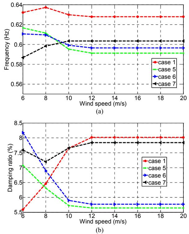
Fig. 8. Influence of wind power ancillary voltage controller parameter  $K_i$  on system inter-area mode. (a) Oscillation frequency. (b) Mode damping ratio
