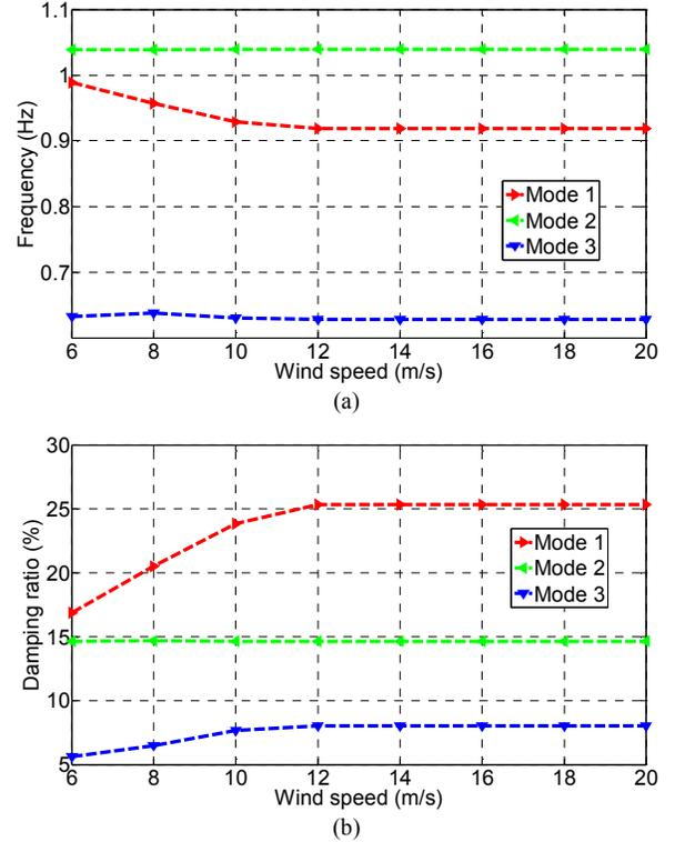
Fig. 6. Influence of wind power integration on system electromechanical oscillation modes. (a) Oscillation frequency. (b) Mode damping ratio
