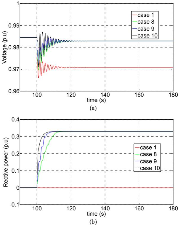
Fig. 4. Ancillary voltage control performance at wind speed 8m/s. (a) Voltage at wind farm point of common coupling. (b) Reactive power output from the wind farm
