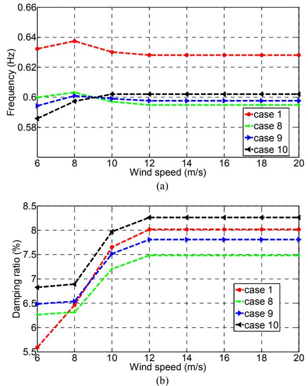
Fig. 9. Influence of wind power ancillary voltage controller on system inter-area mode. (a) Oscillation frequency. (b) Mode damping ratio
