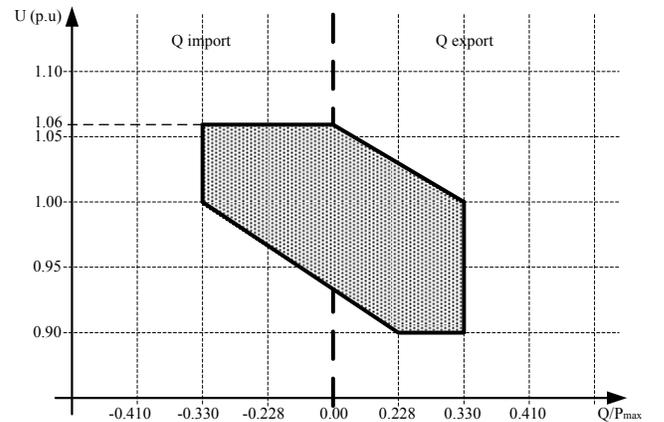
Fig. 1. The requirements for voltage control range for wind farms with output power greater than 25MW
