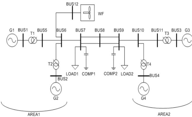
Fig. 3. The two area test power system with a large wind farm
