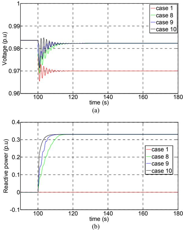
Fig. 5. Ancillary voltage control performance at wind speed 16m/s. (a) Voltage at wind farm point of common coupling. (b) Reactive power output from the wind farm
