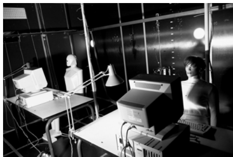
Figure 2. Furnishings and heat load in the full-scale room. The manikin designated A is located on the right side and the manikin designated B on the left side in the picture.
