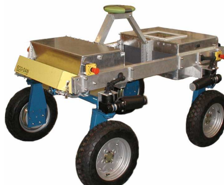
Figure 1. The API II robot. The dimensions of the robot are 150cm (length) by 100cm (width) by 107cm (height). It weighs 226.5kg.
