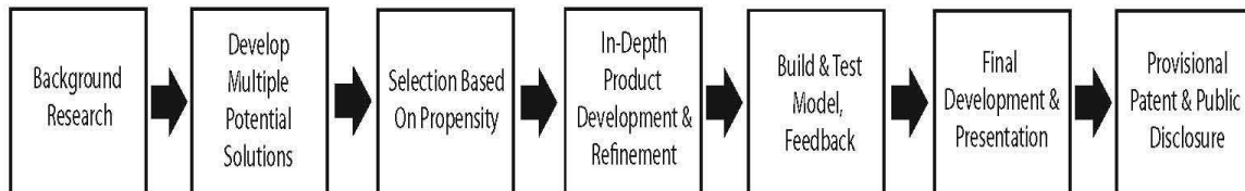
Figure 1: Initial linear progression of product design process
