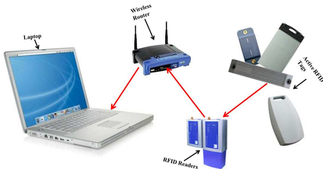
Figure 1: Typical Active RFID Tags and Reader Configuration
