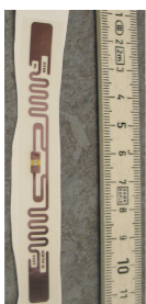
(b) The utilized passive UHF tag. with the coupling element (black) and the tag.
