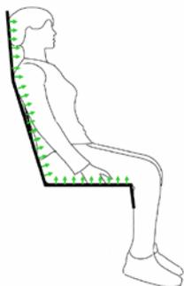
The openings could be formed as bands in the chair or parts, especially in the upper part close to the face regions. The use of textile as supply openings is known in room air diffusion, see the figure.
