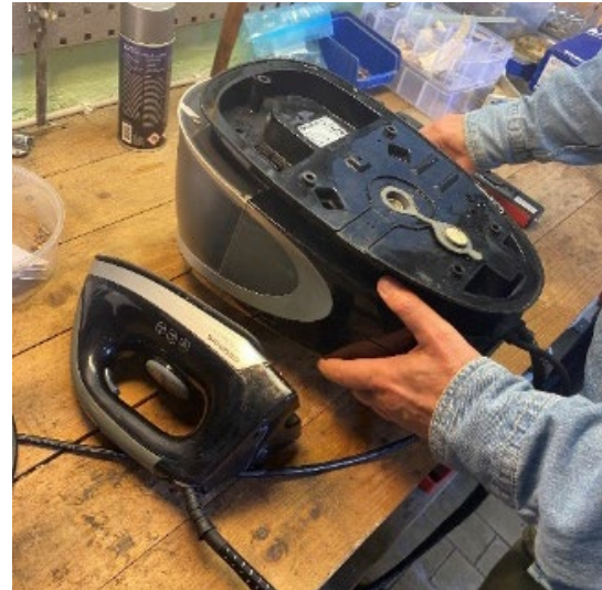
Figure 9. Declogging of a steamer
