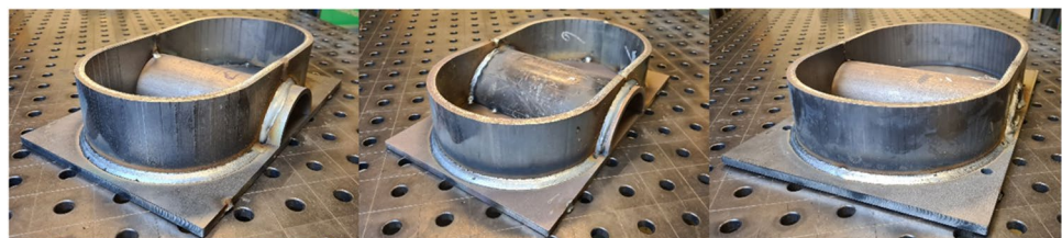
Fig. 12 Resulted weldment following the automatic programming of the welding robot used at the case company. From left to right: Item 1, Item 2 and Item 3, based on the design parameters displayed in Table 2
