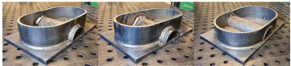
Fig. 9 Resulted weldments following the automatic programming of the welding robot used in laboratory. From left to right: Item 1, Item 2 and Item 3, based on the design parameters displayed in Table 2
