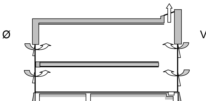
Figur 4. Princip for naturlig ventilation.
