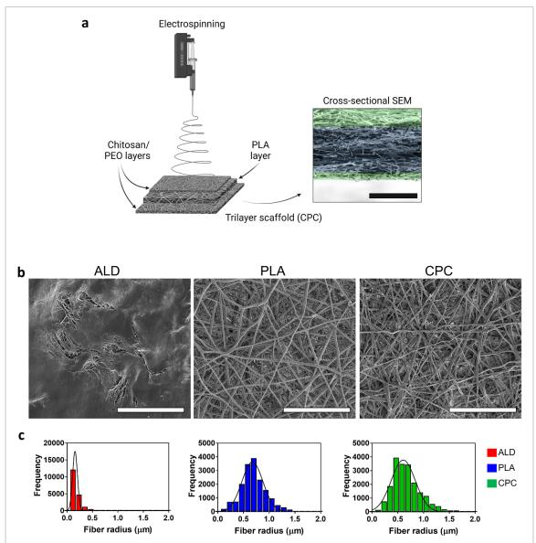
**Figure 1.** (a) Electrospinning set-up for preparing trilayer scaffolds. The schematic illustrates the electrospinning process used to prepare the scaffolds. Scale bar denotes 500  $\mu$ m. (b) SEM images of Alloderm (ALD), poly(lactic acid) scaffold (PLA), and top layer of the trilayer chitosan/PLA/chitosan scaffold (CPC). Scale bar denotes 50  $\mu$ m. (c) Histograms displaying the fiber diameter of the different scaffolds.
